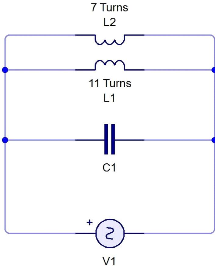
Basic MrPreva schematic where L1 (11 turns) and L2 (7 turns) are wound on the same torroid core
