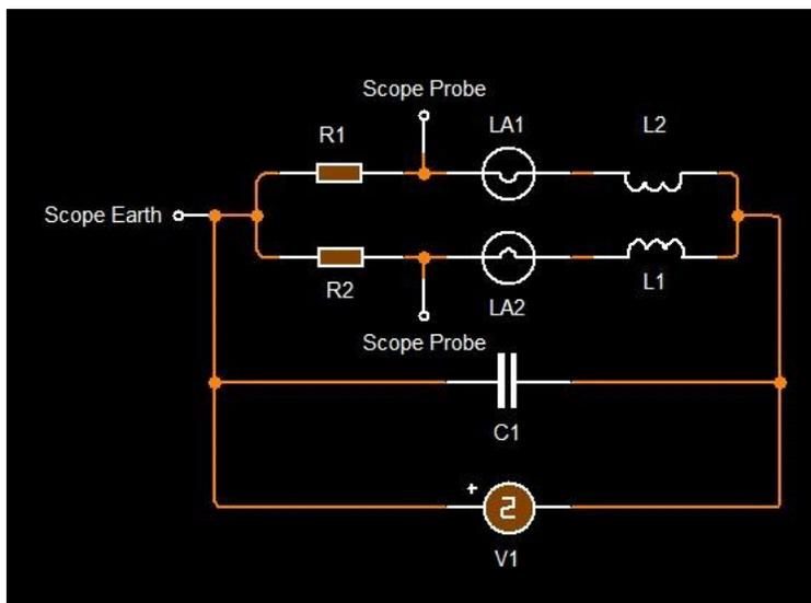
NOTE: C1 and V1 are now in parallel with the series combination of | R1 - LA1 - L2 | and in parallel with the series combination of | R2 - LA2 - L1 |.
